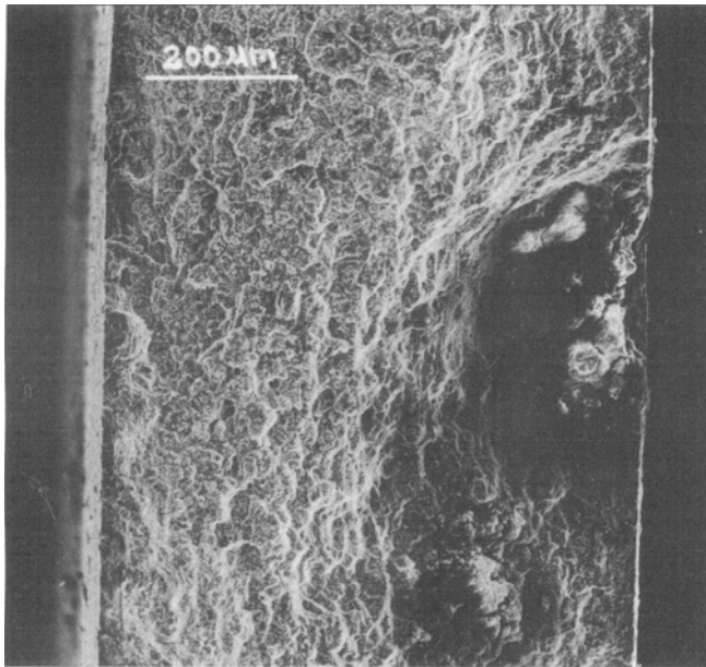
Fig. 17 Scanning electron micrograph of the same specimen in Fig. 15, showing secondary intergranular corrosion on the specimen surface
